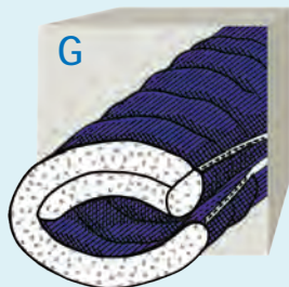
G Continuous Baffle w/ passive top collar & draft tube: Megalite, Monolite, Flylite
